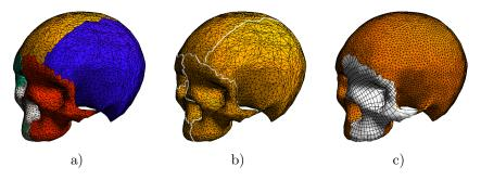
Figure 1: Remeshing algorithm for a skull geometry. a) Initial triangulation (G = 2, NB = 0), b) Remeshing of the lines at the interfaces between partitions, c) Computation of a harmonic map for every partition and remeshing of the partitions in the parametric space.
